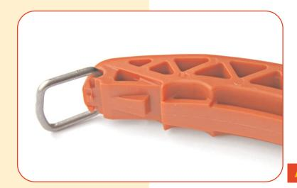
If necessary push firmly with the backside of the comfort tool on the clip as shown.
