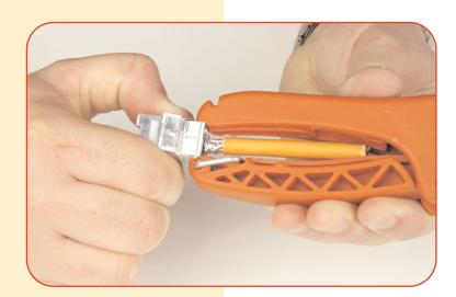
While pressing the comfort tool pull laterally on the connector body until it is removed from the wire organiser.
